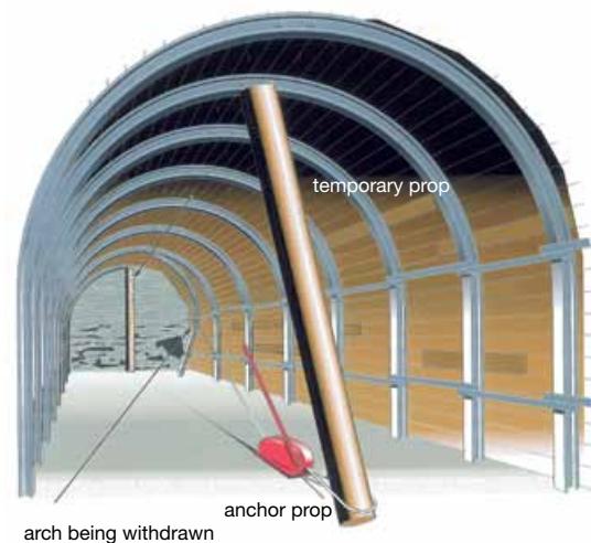
Figure 7c Drawing off in an abandoned roadway
