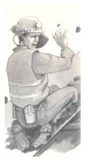
Figure 18 Potential danger of manriding with mineral on steep gradients
