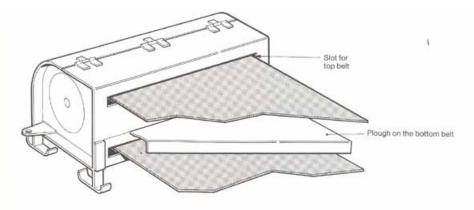
Figure 20 Belt conveyor return end nip guard
