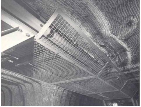
Figure 9 Guarding at a conveyor underpass at a non-coal mine
