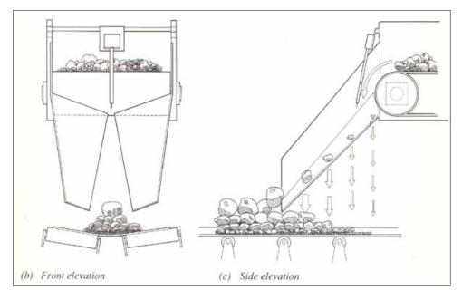
Figure 12 Chute designed to counteract blockages and belt wear
