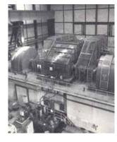
Figure 1 Cable belt conveyor drive-head at Gascoigne Wood Mine, Selby
